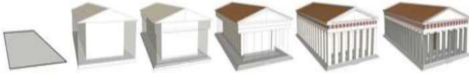
Figure 2. grammar-based modeling identifying rules by generating more and more details that iteratively improve a model.
